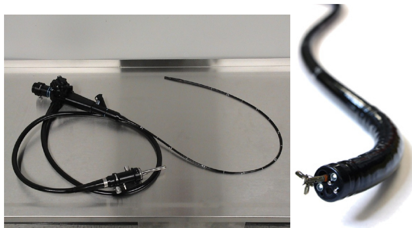
Overview of a standard flexible endoscope (left) and view of the distal part with the camera, optical fiber illumination and operating channel with biopsy clamp inserted.
