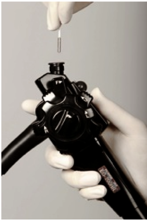
Insertion of a confocal miniprobe into the operating channel of a standard endoscope.
