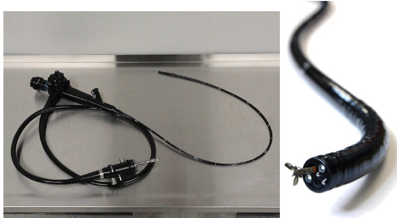
General view of a standard flexible endoscope (left) and view of the distal end with the camera, illumination fiber optics and operating channel, in which a biopsy forceps is inserted
